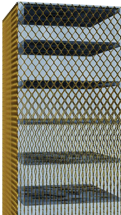
Fig.9.62 – An example of a tower's skin with an increasing size variation along its height.
