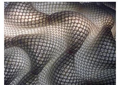
Fig.2.12 – 3D Spacer Textile Composites by Nico Reinhardt (source: www.achimmenges.net/ )
