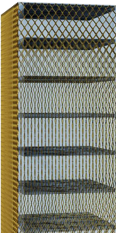
Fig.9.64 - An example of a tower’s skin with an attracted size variation: the attractor-point is placed approximately in the facade’s center.
