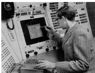
Fig.3.8 - Ivan Sutherland's Sketchpad console, 1962. Sketchpad is operated with a light pen and a command button box (under left hand). The four black knobs below the screen control position and scale of the picture (source: www.mprove.de )
