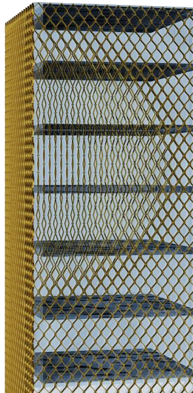
Fig.9.65 - An example of a tower’s skin with an attracted size variation: the attractor-point is placed on the facade’s left side.
