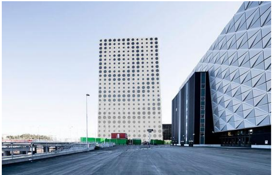
Fig.9.16 - An example of the Quality Hotel Friends facade produced by us: with 13X25 windows, the attractor point is (15 0 60) and the magnitude is 4.
