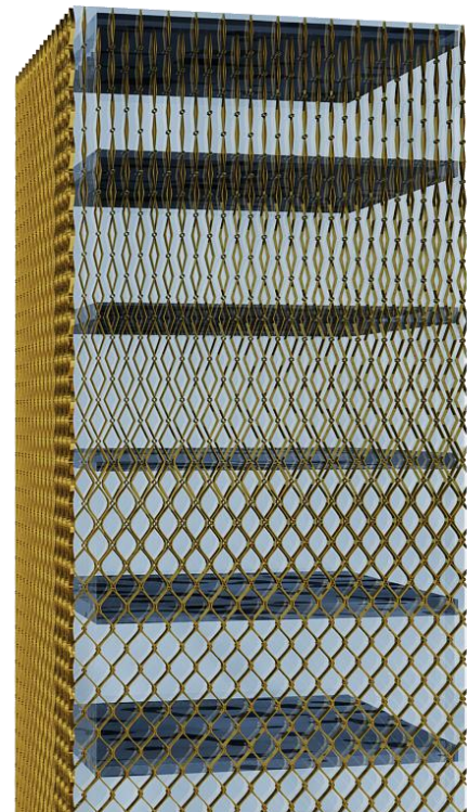
Fig.9.63 - An example of a tower's skin with a decreasing size variation along its height.
